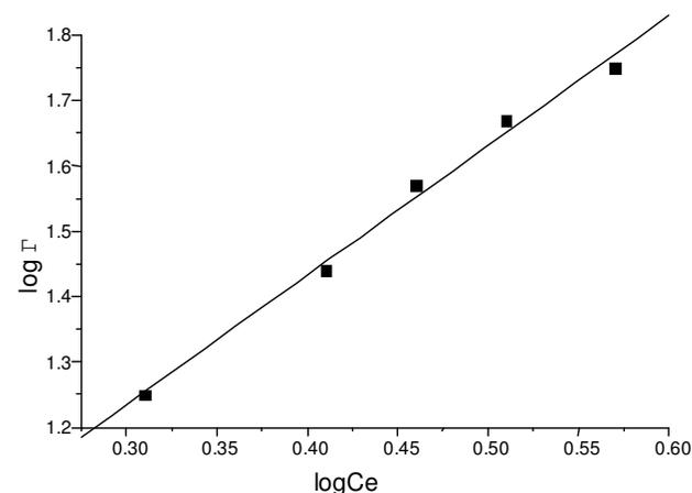
Figure 2. The linearized Freundlich adsorption isotherm of Pb(II) using maize leaf.
